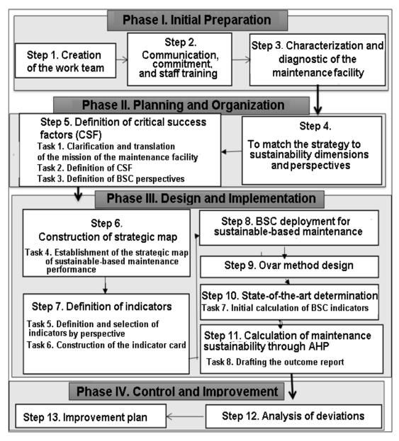
Fig 1. Procedure for BSC implementation in sustainable-based maintenance performance management in plastic transformation factories.
