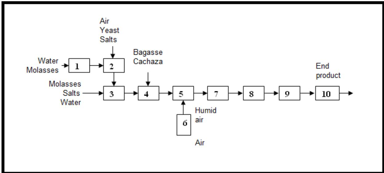
Fig. 1. Box Diagram. 1) Dissolution, 2) Submerged Fermentation, 3) Mixing, 4) Culture media mixing, 5) Solid-state fermentation, 6) Humidifying, 7) Drying, 8) Grinding, 9) Pressing 10) Packaging
